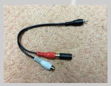
Locate the cabinet speaker RCA cable on the back of the I/O control box. Unplug this cable from the I/O control box.
