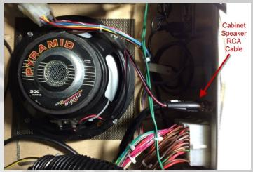
Locate the Aux out cable on the back of the I/O box. Unplug this cable. This cable will connect to the cable going to the isolation transformer mounted next to the 3.5mm Aux out jack on the back.
