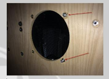
Line up the speaker screen with the two bolts sticking up into the cabinet (from the previous step) Remove the screw holding the nylon cable clamp in place so we can make room for the lower speaker ring. Leave the clamp on the cable!
