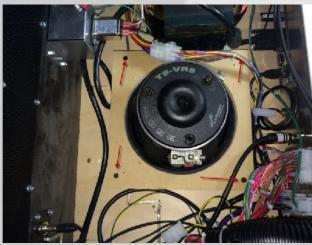
Remove the cover from the I/O Control box. Slide the cover back enough to expose the Amplifier card.
