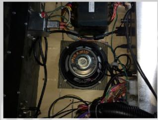
Leave the screen in place. The screen has four holes on it that need to line up with the four holes in the cabinet.
