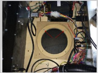
Remove the two screws from the bottom of the cabinet T-nuts and use them to fasten the lower speaker rings two remaining locations.
