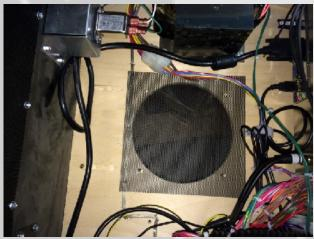
Using two of the removed screws, thread the screws into the T-Nuts on the bottom of the machine as shown. The screws are inserted from the bottom to keep the screen aligned.
