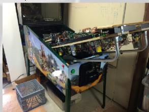
Remove the four screws from the existing speaker. Unplug the cable from the speaker to the connector on the I/O box.
