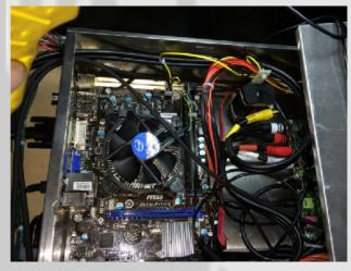
Remove the yellow cable from the amplifier. The yellow cable should be completely disconnected from both ends and taken out of the machine. Insert the RCA cables into the Cabinet speaker outputs on the amplifier board.
