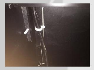
Continue to route the headphone audio cable along the wire harness. Secure the cable in the white cable clamps. The cable will end up at the coin door.
