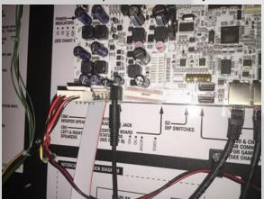
Route the cable into the cable harness clip as shown. It may be a tight fit now that you have two cables going through the clip but it will fit.
