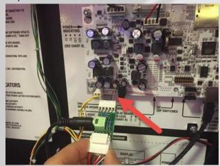
Plug supplied Pinnovators 3.5 mm 12ft cable from the subwoofer cable kit into the 3.5mm green jack on the Back Box Board.
