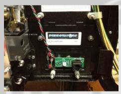
Route the PP4MAC remote cable over the top of the coin slots as shown. Route it down to the system control panel buttons. *NOTE: The three color cable is now a flat three color ribbon cable.*
