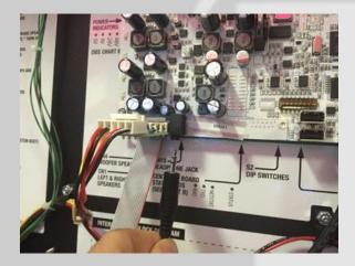
Make sure it is fully inserted into the jack.
