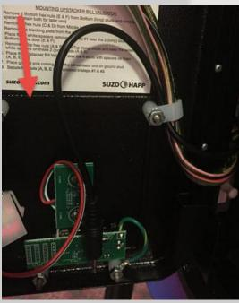
Insert the end of the 3.5mm headphone audio cable into the 3.5mm connector on the PinPAC4 front control panel as shown. The connector is on the front of the control panel PCB. We did this to keep the 3.5mm cable as close as possible to the plate to keep it sleek looking!
