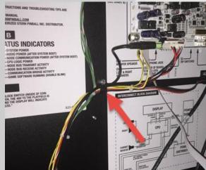
Run the sub cable down through the bottom of the back box and into the main cabinet.
