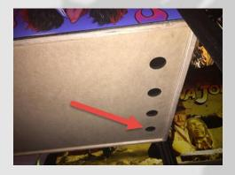
Finally, route the 3.5mm sub cable out the vent hole. Use the included Velcro tie to secure the cable to the leg of the pinball machine.
