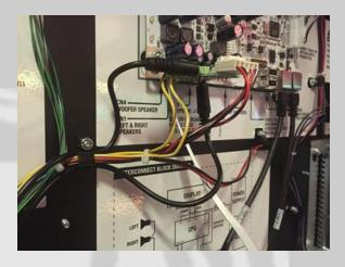
Feed the remaining cable down the bottom of the Back Box and into the cabinet.
