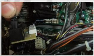
Insert the Back Box Board into the speaker connectors on the sound card as shown below. Make sure it's fully inserted and aligned properly. ALIGNMENT is CRITICAL! You may damage your sound board if the connector is not properly aligned. Check it twice!
