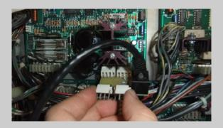
Insert the original Speaker cables on to the pins of the Back Box Board. Note: the connectors can go on either set of pins without causing damage and will function properly.
