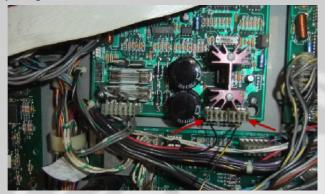
Plug supplied Pinnovators cable into the RJ45 jack on the Back Box Board Connector.
