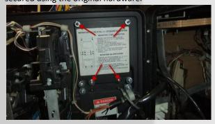
Insert the PinPAC8-PinSound plate as shown below. Position the ESD ground wire (the green wire) under the nearest available threaded stud. Fasten with the original hardware.
