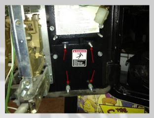
Insert the PinPAC plate as shown below. Position the ESD ground wire (the green wire) under the nearest available threaded stud. Fasten with the original hardware. (Note: This picture shows the cable installed but we will install at a later step.)
