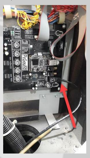
Feed the remaining RJ45 cable down the bottom of the Back Box and into the cabinet.
