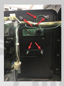
Install the PinPac to PinSound adapter cable as shown below.
