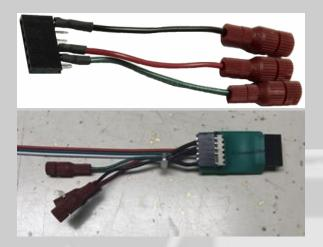
This adapter uses three Posi-Tap connectors. The Posi-Tap connectors will be used to cleanly splice into the button signals for the up and down volume control.
