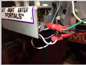
Your Posi-Tap adapter will plug into the connector board at the end of the MAC cable as shown below.
