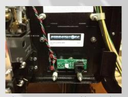
Route the PP8MAC remote cable over the top of the coin slots as shown. Route it down to the system control panel buttons. *NOTE: The three color cable is now a flat three color ribbon cable.*
