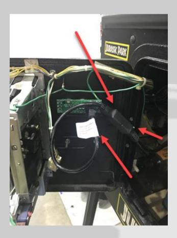
attached to the coin door. The PinPAC plate will fit Stern coin doors.
