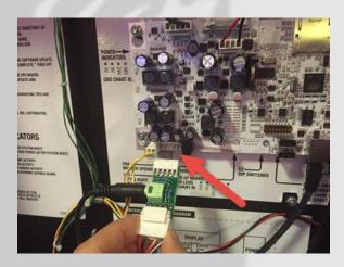
Insert the original Speaker cable on to the pins of the Back Box Board.
