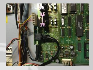
Using the 12 foot 3.5mm to 3.5mm supplied cable, poke the cable through the air vent located above the main CPU board as shown below.
