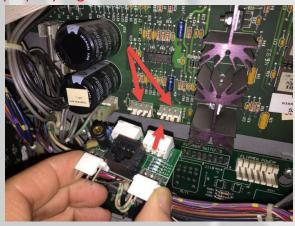
Note: The PINsub\_DCS kit will not have the black RJ45 connector loaded so you will not have an RJ45 cable. The cable is part of the Pinnovators headphone kit.
