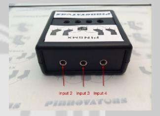
The levels of the four machines can be fully adjusted to your liking by using a small screwdriver and inserting it in the holes on the top of the box. Be carful when turning the controls! Do not force them beyond their end points. The controls are robust but delicate.
